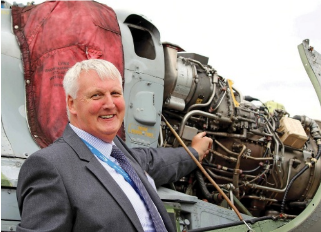
Trevor Jackson of SAE ITC explains to guests that the Rolls-Royce GEM engine on this Lynx helicopter is covered in "standard parts" made to the SAE-ITC drawing standards.
